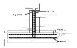
10'-0" FROM GRADE TO TOP OF WALL REINFORCING IS ESTIMATED 77 SQFT AREA = 2.85 CU YDS CONCRETE/FT OF WALL (10) #6, 12' OF #6 = 22FT X 1.5LB/FT = 33LB/FT OF WALL (54) #9, 55' OF #9 = 109FT X 3.4LB/FT = 374/FT OF WALL
